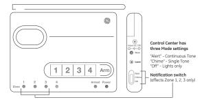
**Zone 4** is designated for detected Alerts only. Use Zone 4 for areas you wish to continuously monitor, but don't want to trigger the alarm (e.g. notification of water leaks, garage door is up, back gate left
